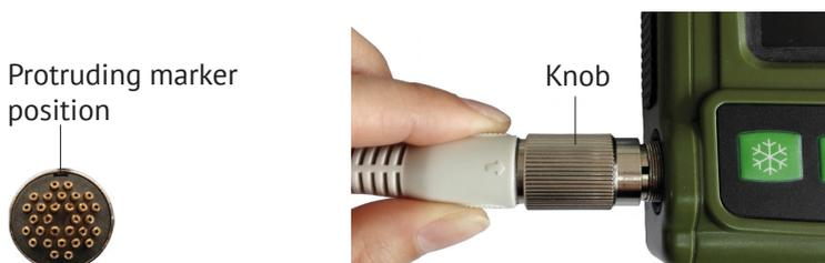
3. After pushed in place, hold the machine with one hand and rotate the knob clockwise with the other hand until the probe is locked.
