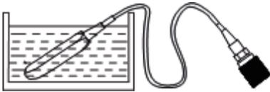
Fig. Immersion disinfection of intra-cavity probe (sketch map)
